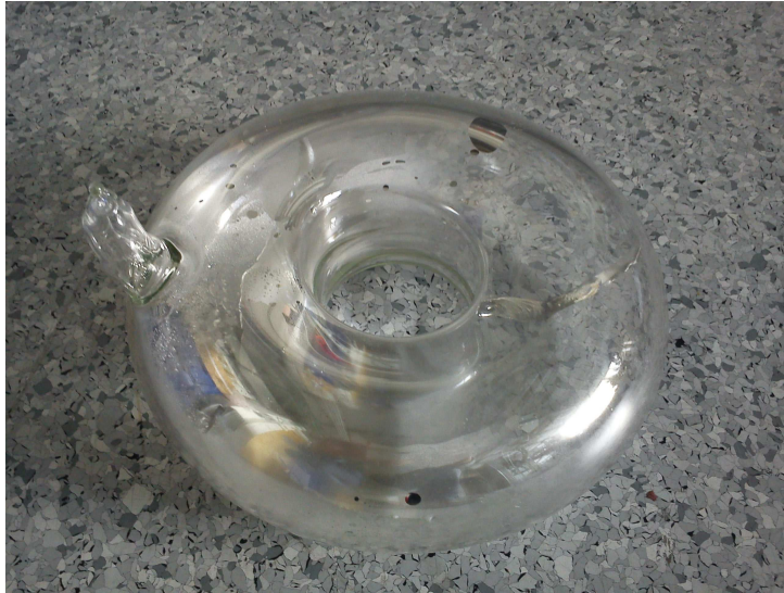
Figure 5. A first doughnut shaped cell for magic PASTIS testing called Homer. This cell is filled with 0.5 bar of ^3\text{He} to make it sensitive to magnetic field gradients. The T_1 lifetime of this cell is 1074 \pm 20 hours. (Color online)
