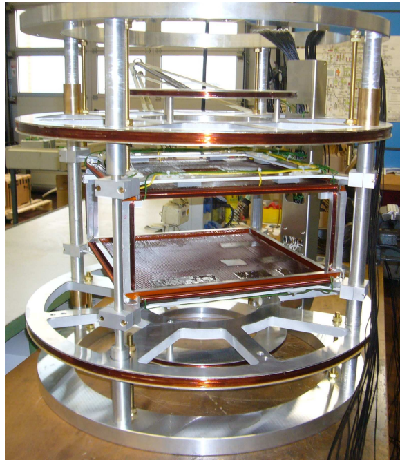
Figure 4. The current status of the magic PASTIS system. The system is now being optimized for the values of currents and fine positioning of coils. (Color online)
