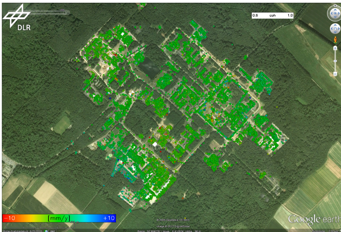
Figure 1. PSI deformation map over FZ Jülich using the descending HRS TerraSAR-X stack.
