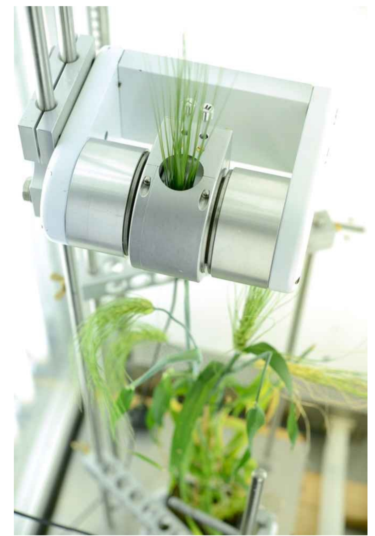
Fig 5: Non-invasive measurements of starch deposition, water content or transport using portable NMR (5)
