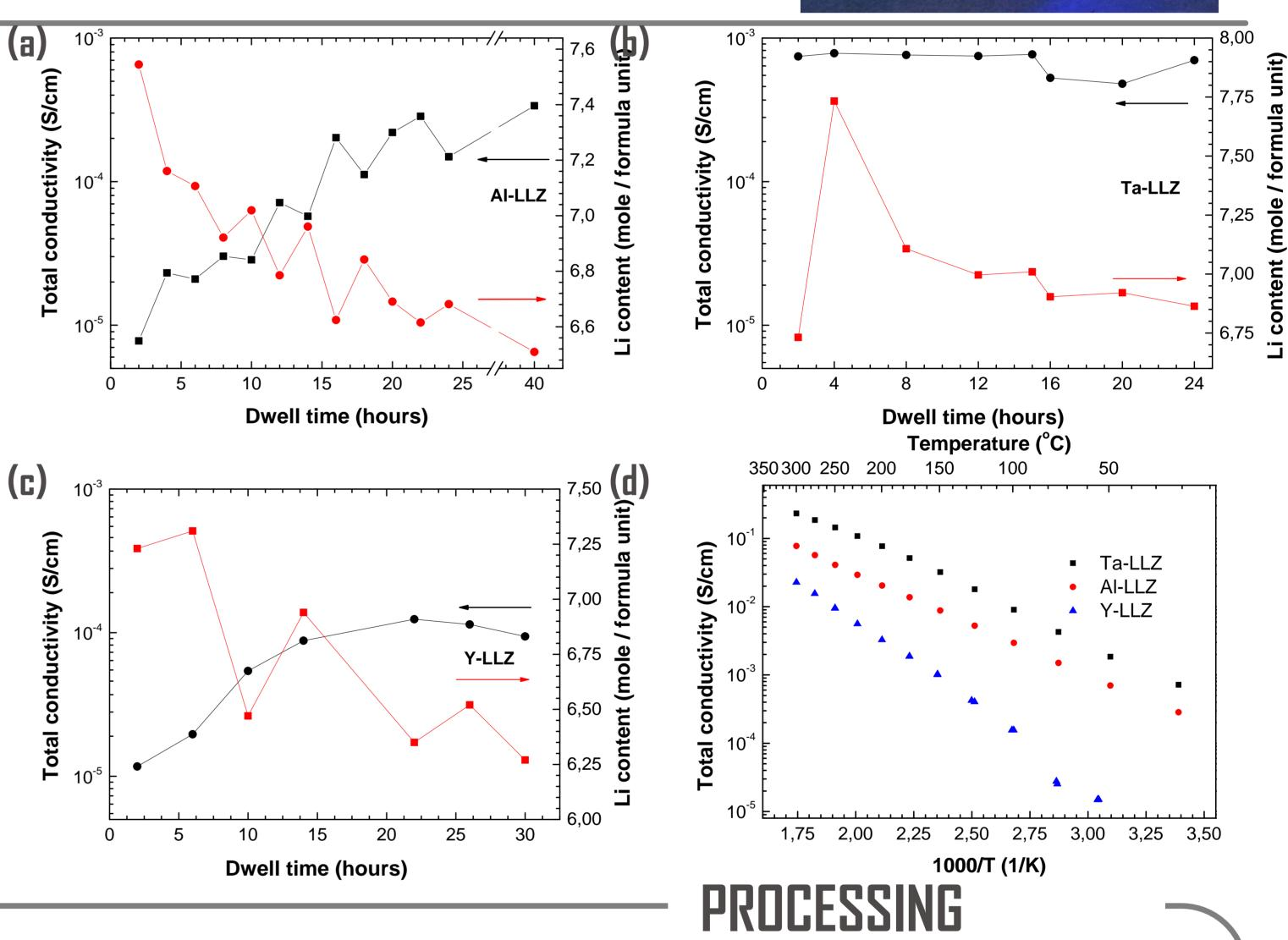
(d) Temperature dependence of the ionic conductivity of AI-, Ta- and Y-substituted LLZ. Ta-substituted LLZ shows the highest total ionic conductivity among the three materials. The total conductivity was derived from impedance spectra (1MHz-1Hz, amplitude: 20 mV/mm, temperature range: 22-300°C).
