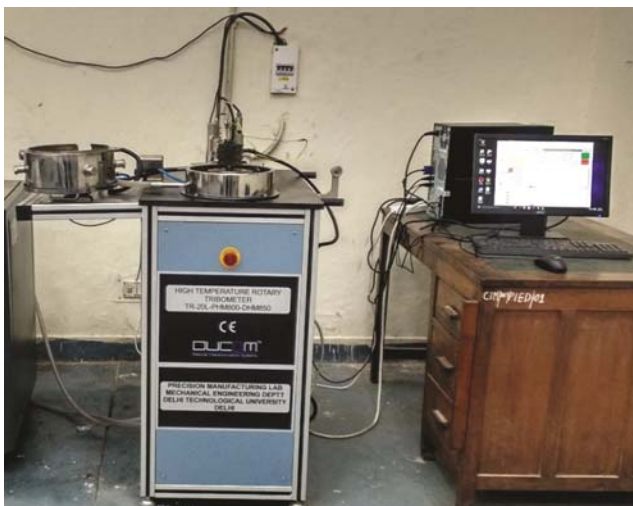
Fig. 1 — Experimentation set-up of used test rig (pin-on-disc).
