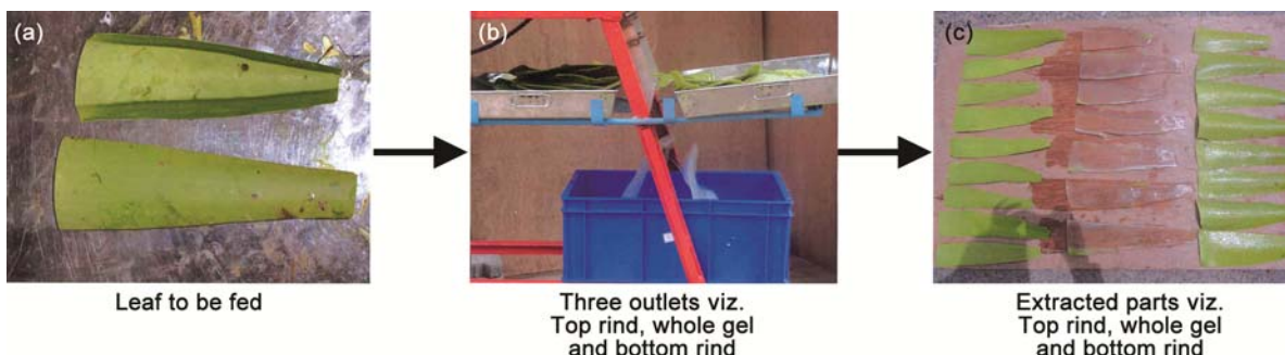
Fig. 3 — Extraction process of continuous feed equipment for aloe vera whole gel extraction: a) Leaf to be fed b)Three outlet viz., top rind, whole gel and bottom rind c) Extracted part viz., top rind, whole gel and bottom rind
