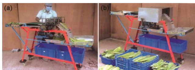
Fig. 2 — Continuous feed equipment for Aloe vera whole gel extraction a) without cover b) with cover
