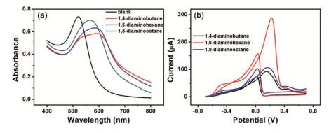
Fig. 4 — (a) UV–visible absorption spectra for the pSC<sub>4</sub>-Au-NPs assembled by 1,4-diaminobutane, 1,6-diaminobexane and 1,8-diaminooctane. (b) CVs of the 1,4-diaminobutane-pSC<sub>4</sub>-Au-NPs (black line), 1,6-diaminobexane-pSC<sub>4</sub>-Au-NPs (red line) (b) and 1,8-diaminooctane-pSC<sub>4</sub>-Au-NPs (blue line) modified electrodes in the presence of 10 mM glucose in 0.1 M NaOH at a scan rate of 50 mV s<sup>-1</sup>.
