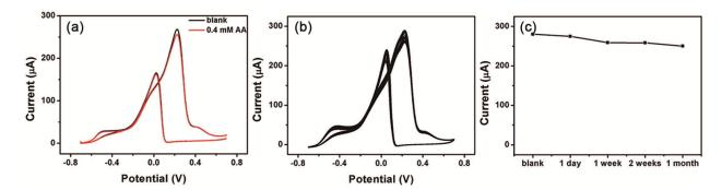
Fig. 5 — (a) CVs at the HMD-pSC<sub>4</sub>-Au-NPs modified GCE in 10 mM glucose in 0.1 M NaOH solution before (black line) and after (red line) the addition of 0.4 mM ascorbic acid. The scan rate is 50 mV s<sup>-1</sup>. (b) Corresponding curves of HMD-pSC<sub>4</sub>-Au-NPs modified electrodes response to different scan times in the presence of 10 mM glucose in 0.1 M NaOH at a scan rate of 50 mV s<sup>-1</sup>. (c) Plots of the electrocatalytic current *vs* time of the modified electrodes.
