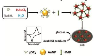
Schematic illustration of the mechanisms for the synthesis of pSC4-Au-NPs, pSC4-Au-NPs aggregation induced by host–guest recognition, and evaluation for electrocatalyst Scheme 1
