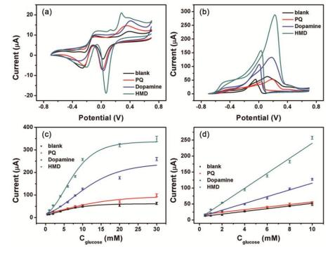
Fig. 3 — CVs of the pSC<sub>4</sub>-Au-NPs, PQ-pSC<sub>4</sub>-AuNPs, dopamine-pSC<sub>4</sub>-Au-NPs and HMD-pSC<sub>4</sub>-AuNPs modified electrodes (a) in the absence and (b) presence of 10 mM glucose in 0.1 M NaOH at a scan rate of 50 mV s<sup>-1</sup>. Linear relationships of the electrocatalytic current of glucose *vs* concentration are shown in plot for (c) 0–30 mM and (d) 0–10 mM of the modified electrodes.
