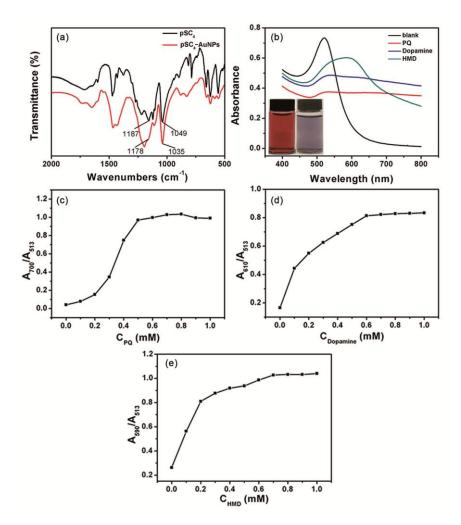
Fig. 1 — (a) FTIR spectra of the pSC<sub>4</sub>-AuNPs, (b) UV-visible spectra for the pSC<sub>4</sub>-AuNPs assembled by PQ (0.5 mM), dopamine (0.6 mM) and HMD (0.7 mM), Plots (c, d and e) for the pSC<sub>4</sub>-Au-NPs assembled by PQ, dopamine and HMD (0–1 mM).
