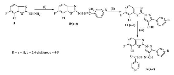
Reagents and conditions: (i) substituted acetophenone, 2-3 drops glacial acetic acid, methanol, reflux, 0.5 h; (ii) POCl<sub>3</sub>-DMF, stir, 60-65°C, 3 h; (iii) isoniazid, toluene, 2-3 drops glacial acetic acid, reflux, 24 h
