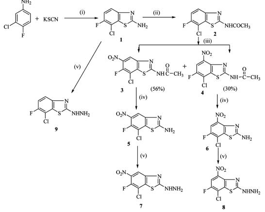
Reagents and conditions: (i) Br<sub>2</sub>, CH<sub>3</sub>COOH, 5°C, stir, NH<sub>3</sub>; (ii) (CH<sub>3</sub>CO)<sub>2</sub>O, reflux 1 h; (iii) conc. HNO<sub>3</sub> and conc. H<sub>2</sub>SO<sub>4</sub>, stir, RT (iv) 70% H<sub>2</sub>SO<sub>4</sub>, reflux, 30 min; (v) NH<sub>2</sub>.NH<sub>2</sub>.H<sub>2</sub>O/ HCl, ethylene glycol, reflux 2 h
