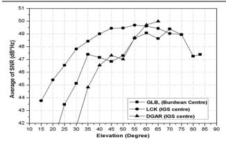
Fig. 7 — Comparison of GPS signal strength variation for the same GPS satellite (PRN #16) from different locations on 20 June, 2018
