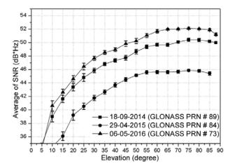
Fig. 3 — Variation of average and standard deviation of signal strength of L1 C/A signal of different GLONASS satellite generations; PRN #89 and PRN #84 (GLONASS M); PRN #73 (GLONASS K)
