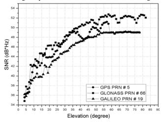
Fig. 1 — Variation of SNR values with increasing elevation angles for GPS, GLONASS and Galileo satellites on 19 September 2014 using JAVAD DELTA G3T receiver
