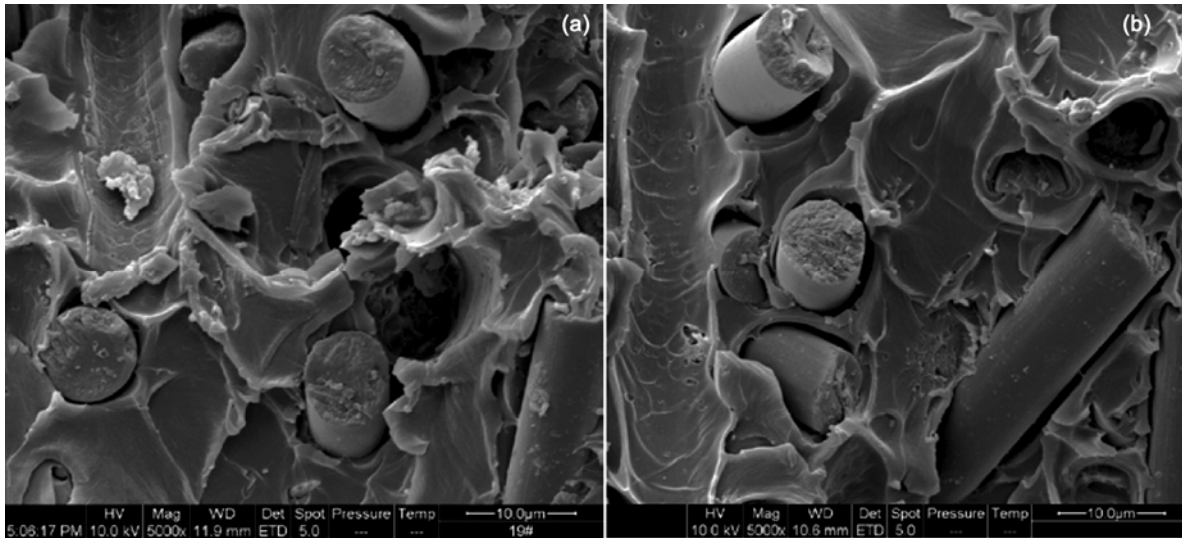
Fig. 6 — SEM morphologies of the fracture surface of composites reinforced with (a) untreated CF and (b) sized CF.
