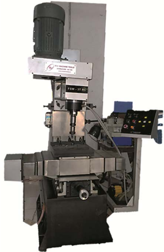
Fig. 1 — Friction stir welding machine (3 tonne capacity).
