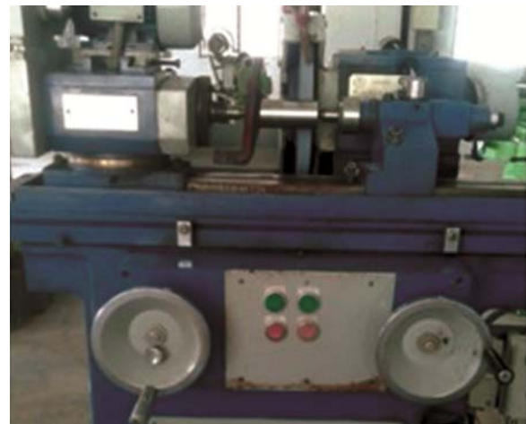
Fig. 1 — Experimental set up for cylindrical grinding.
