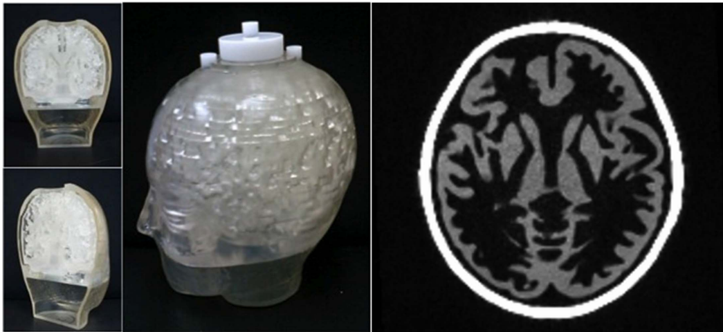
Figure 2. Left: Photographs of the Iida brain phantom used in this study. On the left, the sections show the elaborate internal structure of the phantom with the putative ‘grey/white matter’ compartments. Right: Transaxial MPRAGE image of the brain phantom with the same slice position as shown in Fig. 7.
