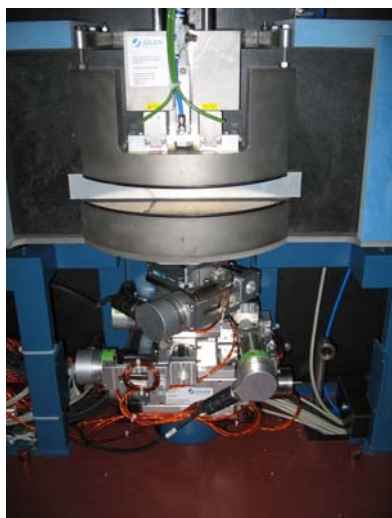
FIG. 2: The monochromator column inside the monochromator shielding (blue part on the right in Fig. 1) with the five axes assembly necessary to move the monochromator crystal according to the desired wavelength. In the upper part of the picture the first instrument shutter called photo-shutter can be seen which consists of a 4 mm B 4 C ceramic plate moved by an air piston. The remaining space in front of the monochromator column is reserved for two apertures and a velocity selector.
