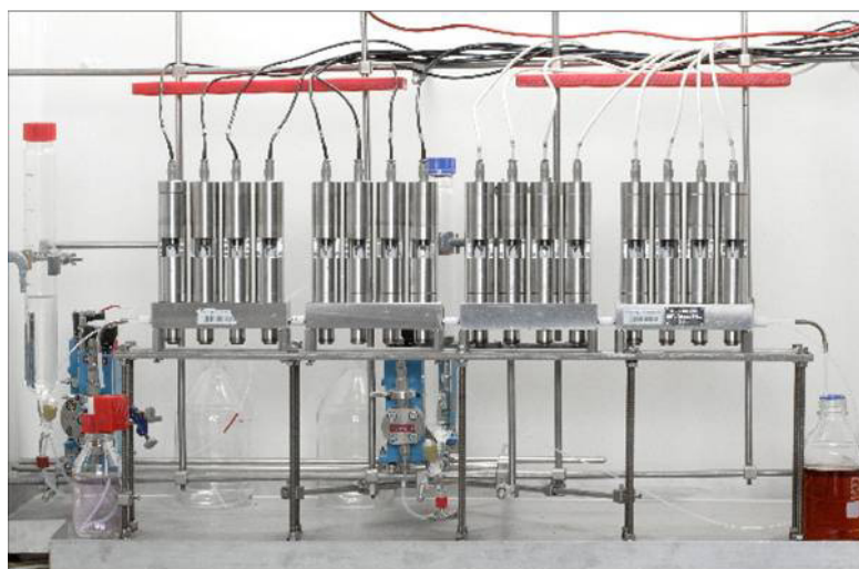
Figure 73. Battery of miniature centrifugal contactors for performing tests in counter-current mode.
