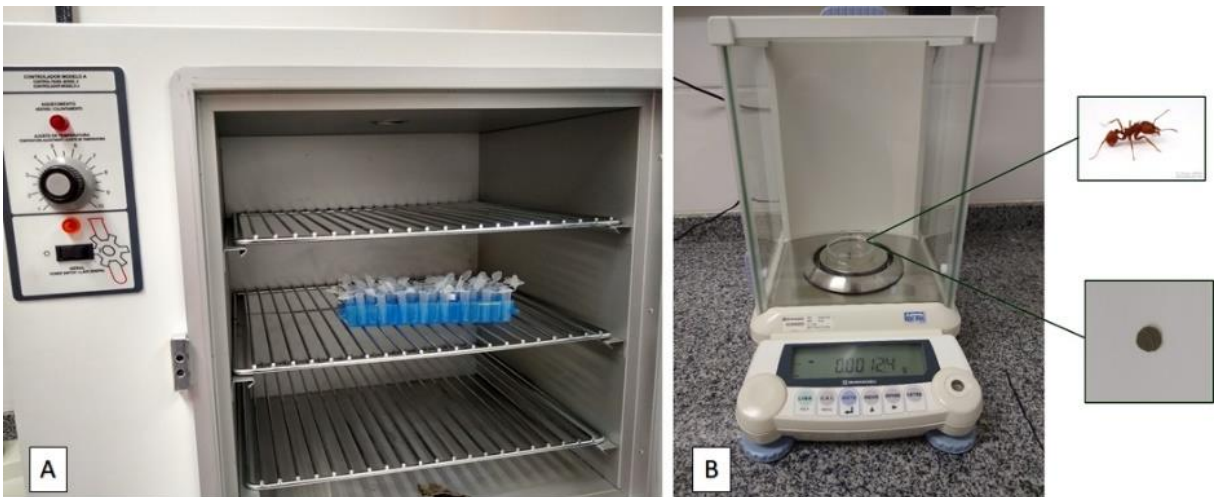
Figure 6 - (A) Oven used for the dehydration of workers and leaf discs and (B) analytical balance used for weighing leaf discs and Acromyrmex subterraneus workers.
