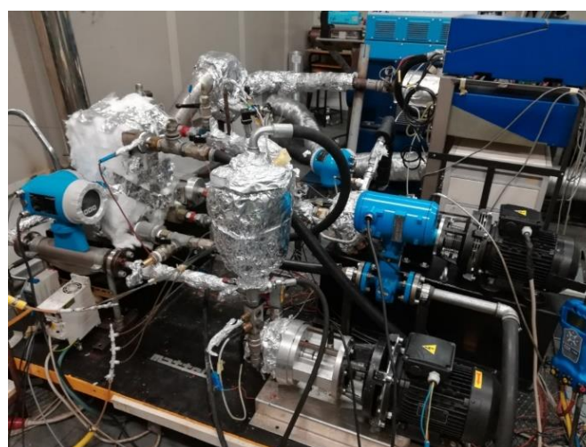
Figure 2. ORC (Organic Rankine Cycle) test rig.
