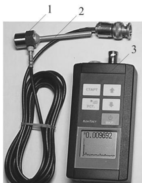
Fig. 2. Instrument for measuring oscillation parameters "Vibrometer 107B": 1 - accelerometer; 2 - probe; 3 - the vibrometer
