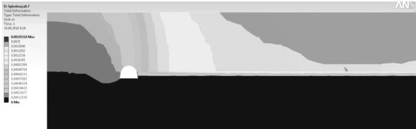
Fig. 1. Total deformations of rock mass in front of the slope face in the process of complete backfilling if height of the rocks being cut is 0.7 m [3]
