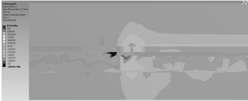
Fig. 2. Vertical stresses in a cross section at 0.5 m distance from a mine working in the process of packing when height of rocks being cut is 0.5 m
