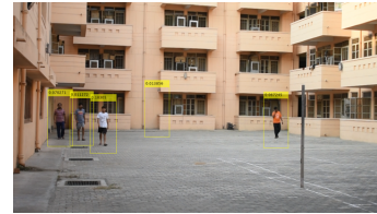
Fig. 4. Person detection using HOG + SVM model.
