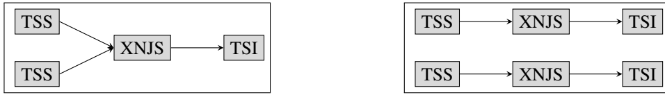
Figure 2. Comparison of the existing (left) and proposed (right) UNICORE architectures. In the new model, each TSS represents its own XNJS.
