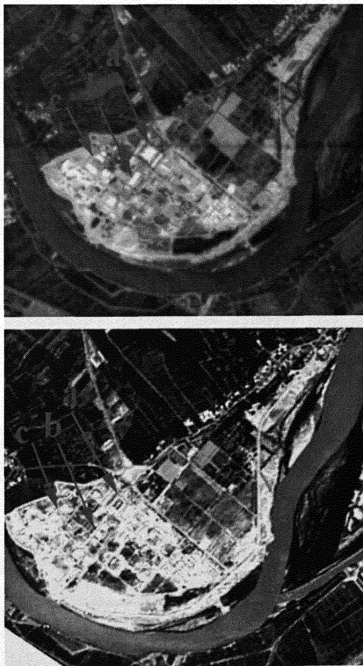
Figure 3.10. Extracts from the full scenes over Baghdad acquired by the Russian KVR-1000 sensor (top) on 27 June 1990 (before the Gulf War) and the French SPOT satellite (lower image) on 12 May 1991. (a) is the site of the EMIS machine housing; (b) an un-identified building which appears to have changed in 1991 (see the lower SPOT image); and similarly changes have occurred at c.
