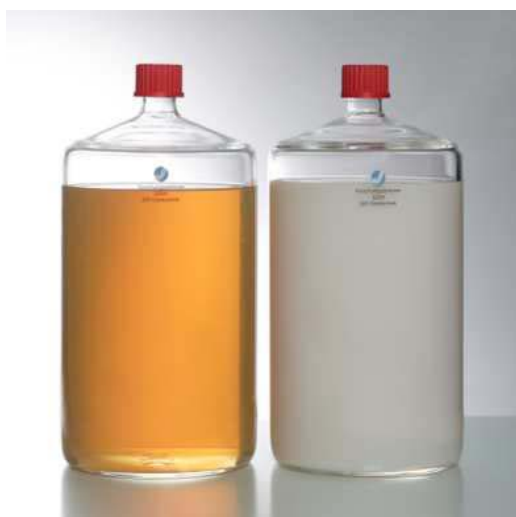
FIG. 2: Microemulsion cleaners with high surfactant content (left) and low surfactant content (right).
