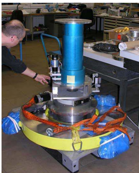
FIG. 3: The sample stage which has been completed with a lifting mechanism to automatically switch between different samples.
