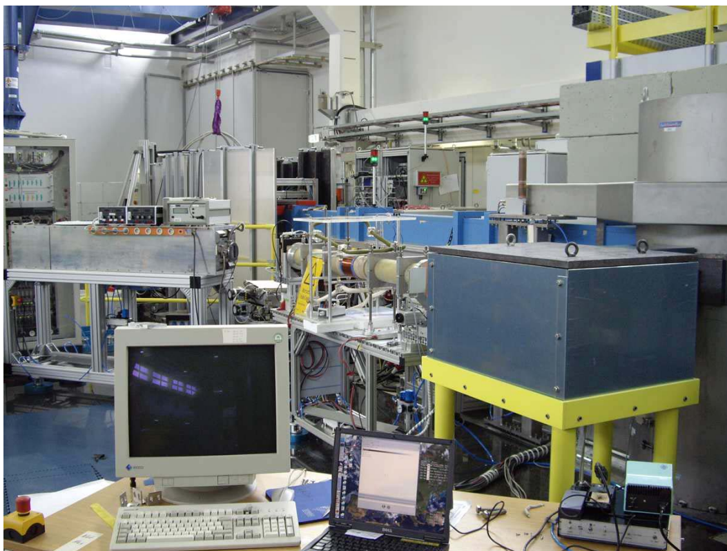
FIG. 2: TREFF@NOSPEC: From the cylindrical shielding of the first monochromator (right) the neutrons are brought to the shielding box of the second monochromator. Then follows the collimation (with the resonance spin flipper coil around the vacuum tube), the sample table and the detector arm (middle left).
