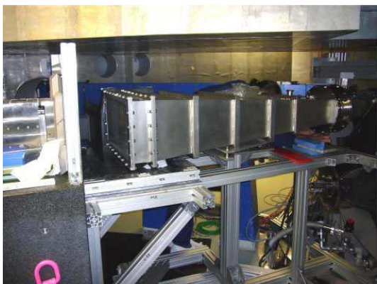
FIG. 2: Newly installed vacuum flight chamber between the PST chopper (right side) and the Doppler monochromator (left side).
