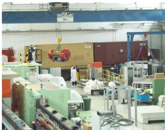
FIG. 1: One of the two main precession coils of the J-NSE spectrometer entering the neutron guide hall
