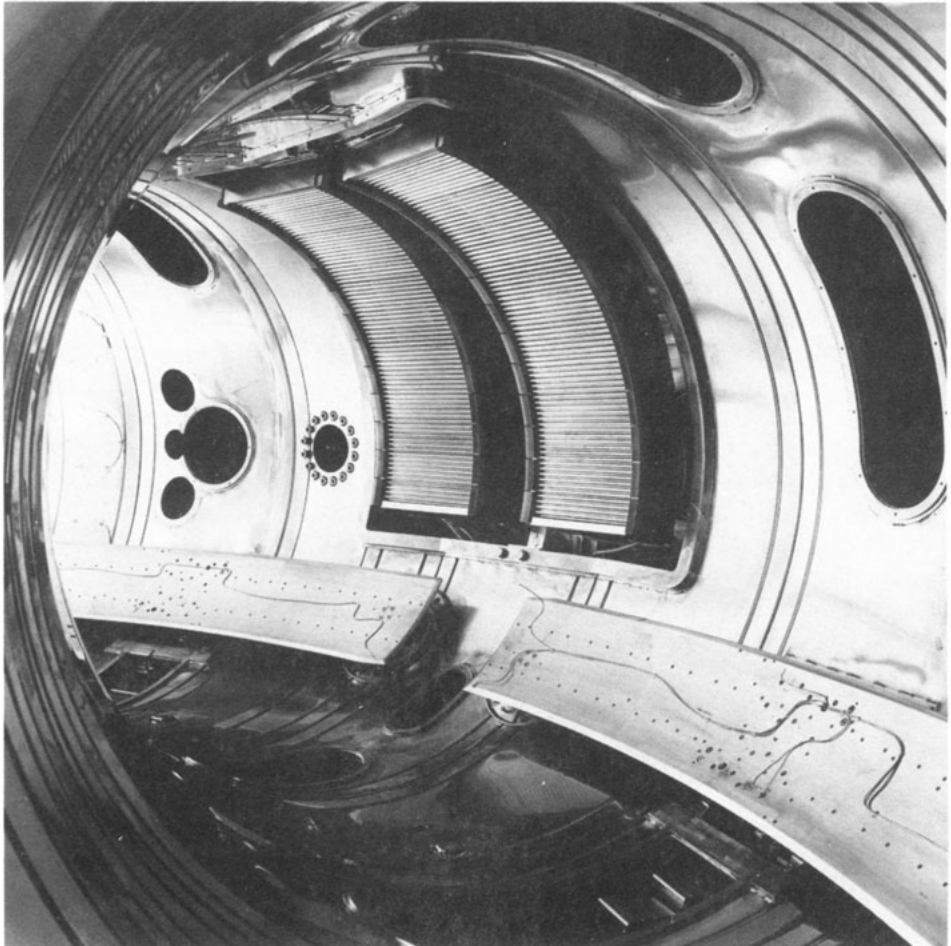
FIG. 1(a).—View of one pair of new movable ICRH antennae installed in the TEXTOR liner. Parts of the toroidal belt limiter ALT II are seen underneath.
