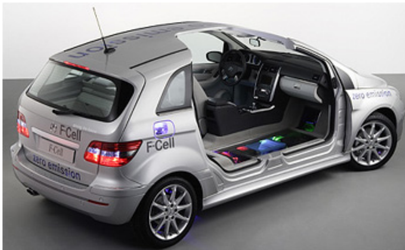
Figure 3: Cross-sectional model with stack.
