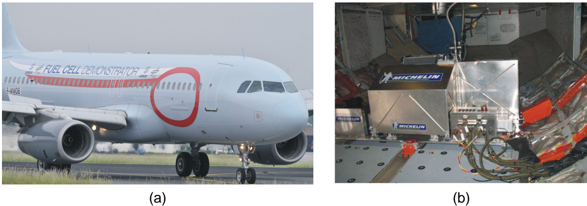
Figure 1: (a): DLR research aircraft A320 (D-ATRA) at Berlin International Air Show (ILA) 2008. (b): Michelin fuel cell system in the cargo area of the research aircraft.
