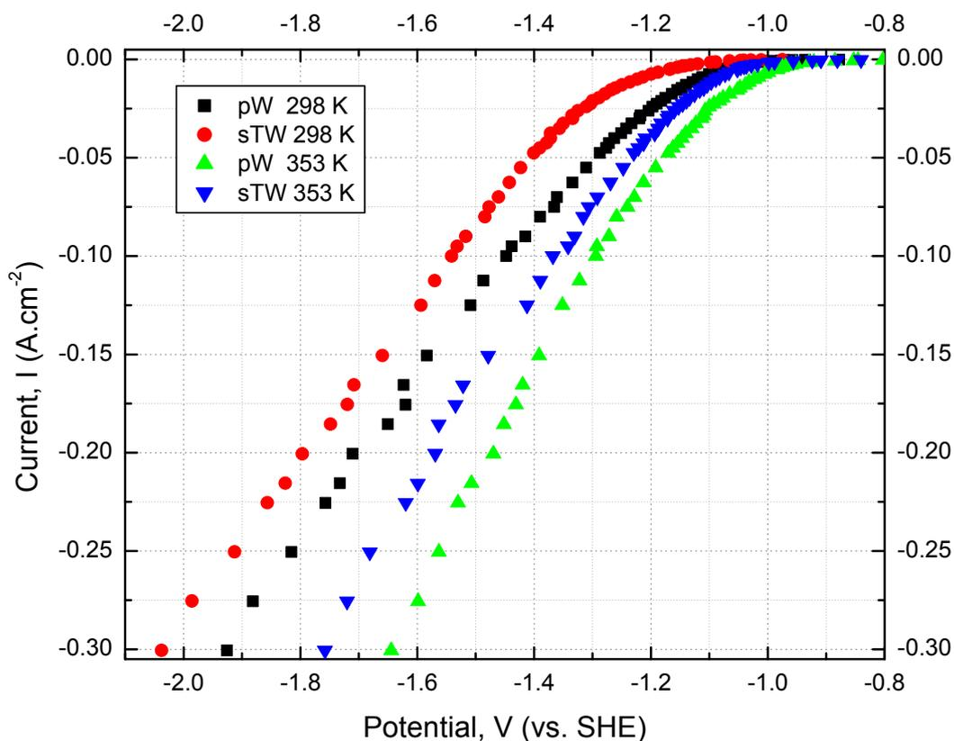
**Figure 1:** Polarization curves of Ni electrode in 1 mol.dm<sup>-3</sup> KOH pure water (pW) and synthetic tap water (sTW) at two different temperatures.
