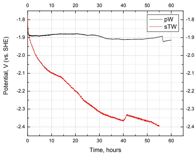
**Figure 5:** Stability test for Ni electrode in  $1 \text{ mol.dm}^{-3}$  KOH pure water (pW) and synthetic tap water (sTW) at 298 K and constant current density of  $0,25 \text{ A.cm}^{-2}$ .
