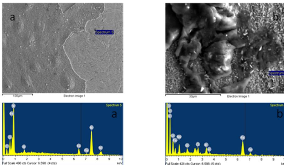
**Figure 2:** SEM and EDX spectrum images of Ni electrode after steady-state polarization in a) pure water + 1 mol.dm<sup>-3</sup> KOH, b) synthetic tap water + 1 mol.dm<sup>-3</sup> KOH.
