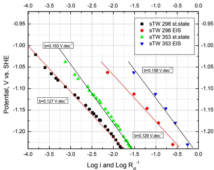
**Figure 4:** Comparison of the Tafel slopes obtained from steady-state and EIS techniques in sTW at 298 and 353 K.
