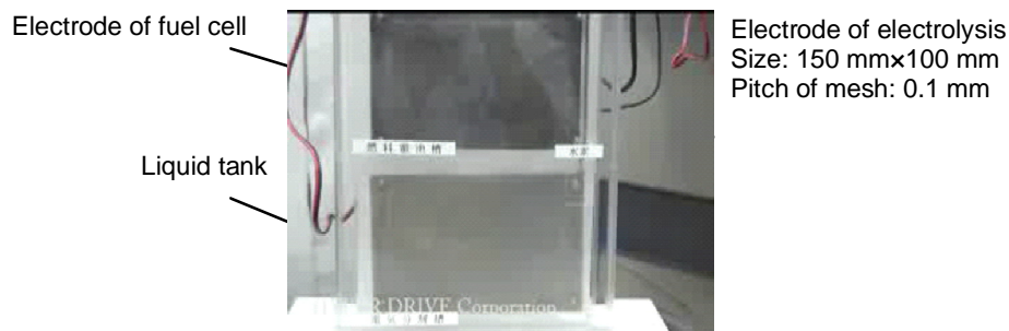
Photo 3: Hydrogen generation equipment by electrolysis.
