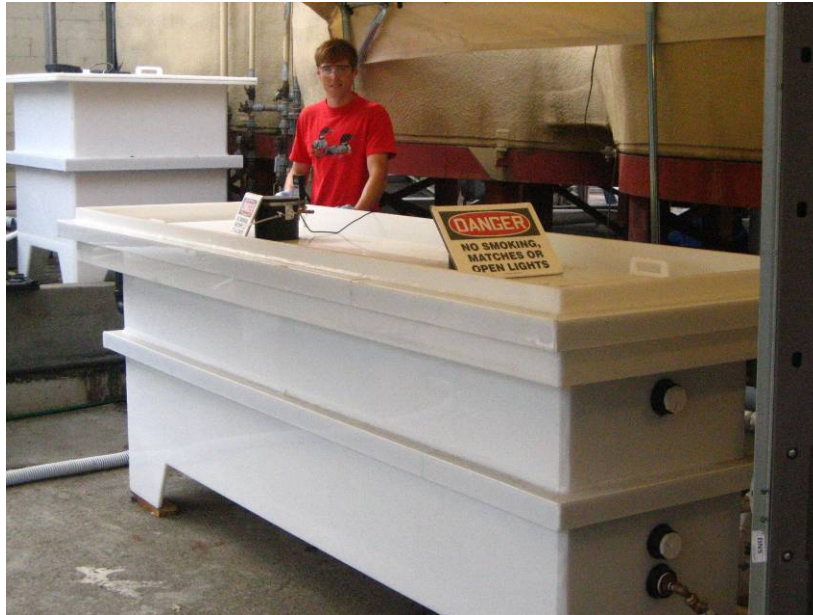
Figure 2: Photograph of a 1000-liter MEC being tested for hydrogen production using wastewater from a winery.
