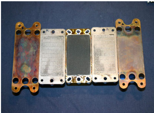
Figure 1: Single cell components after 3000 hrs of operation.
