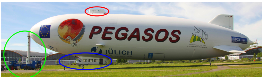
Figure 2.3.: Airship Zeppelin NT as used during the 2012 PEGASOS mission. The Top-Platform is highlighted in red, the gondola including a nose-boom in blue, and the Mast-Truck in green.
