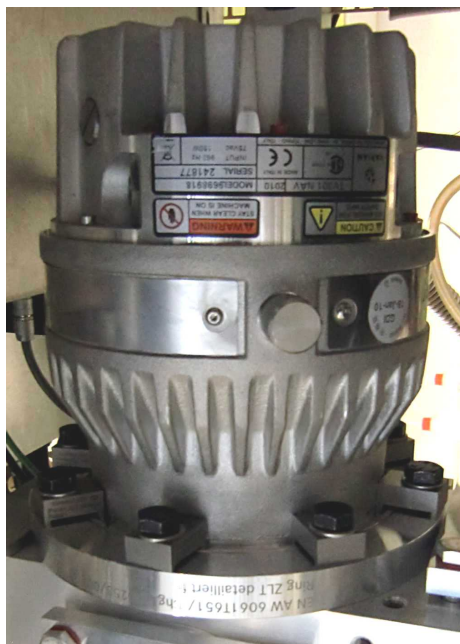
Figure 2.11.: Photograph of a Varian TV301 Navigator turbomolecular pump and its mounting on the AMS PToF chamber. A ring around the base of the pump holds eight clamps pressing the pump down, of which four are fixed to the PToF chamber, the other four are fixed to the ring itself.
