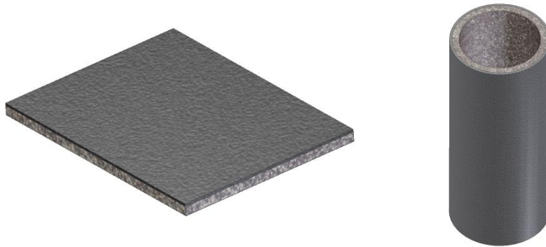
Figure 4–12: Illustration of planar and tubular membrane assembly.
