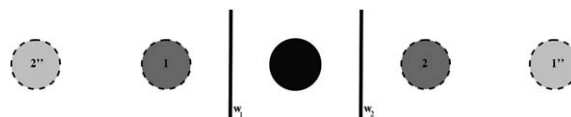
Fig. 11 Schematic diagram of the reflection method used in our calculations. With solid lines, the actual walls and the central colloid; with dashed lines the corresponding images.
