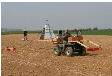
Figure 2. Far-field GPR (horn antenna linked to a VNA, D-GPS device, and a PC), near-field GPR (on the back), and EMI sensor (on the front) mounted on a quad to measure soil dielectric permittivity and apparent electrical conductivity.
