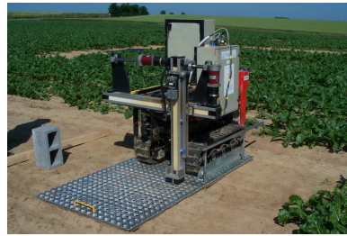
Figure 3. Fully automated penetrometer used for the soil strength measurements [2].
