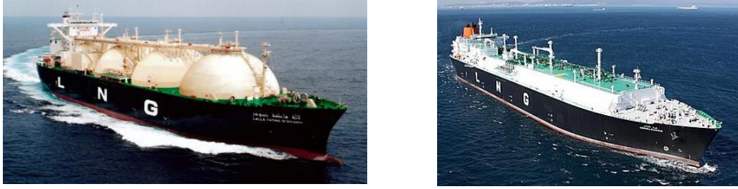
(a) Spherical tank or MOSS technology (b) Prismatic tank or membrane technology
