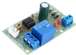
Gambar 2. Sensor Water Level Control
