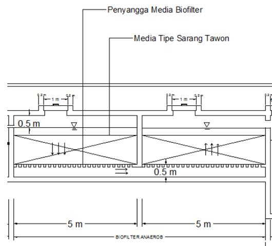
Gambar 7. Biofilter Anaerob
