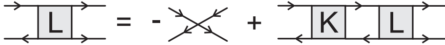
Figure 1. Graphical representation of the Bethe-Salpeter equation for the response function in the ph channel.
