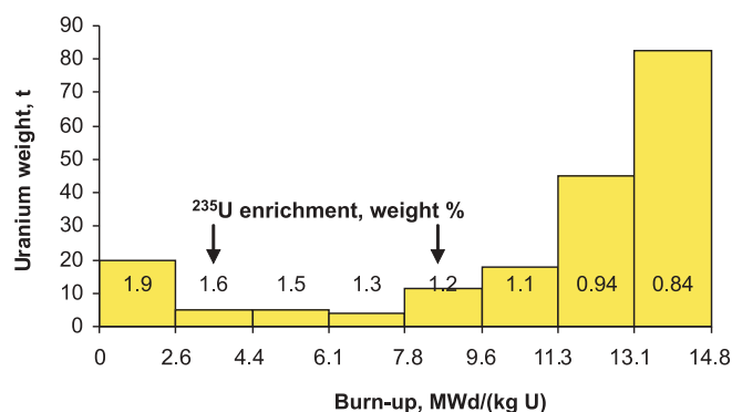
Fig. 1. Burn-up distribution and ^{235}\text{U} enrichment in fuel fragments of the damaged Chernobyl reactor, calculated data by Begichev et al. [1].
