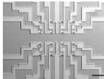
Fig. 2. Micrograph of the sensitive FET surface. The scale bar represents 200\mu\text{m} .
