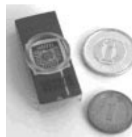
Fig. 1. FET-based microelectronic device. The sensitive silicon chip is mounted on a zero-force socket. A glass ring glued to the socket forms a petri dish for cell-culture on the device surface.
