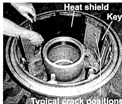
Fig. 1. Photograph of an Boeing 747 aircraft wheel rim. Typical position of inside cracks next to keys are indicated. They are not accessible from the inside because of the heat shields (some are removed for the photo).
