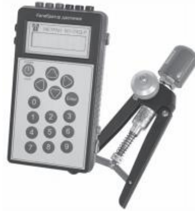
Fig. 6. Portable Metran 501-PCD-R pressure Calibrator
