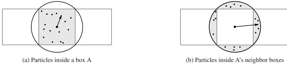
Figure 2.15.: In general it is not possible to set ws to zero, since neighboring boxes may have particles overlapping with the multipole expansion of a neighboring box. However, the convergence of the expansion demands separation. Therefore, next neighbors must not interact via a multipole expansion.
