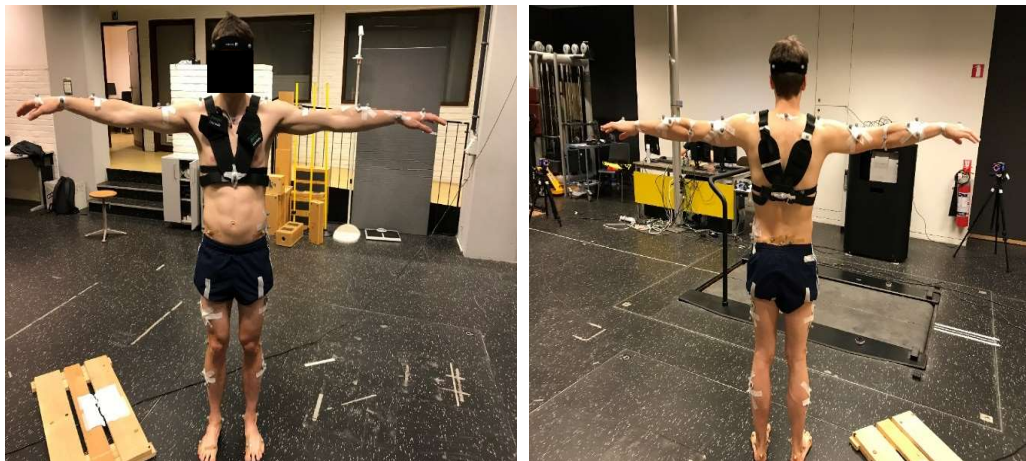
Figure 44. Anterior and posterior views of the full body marker set with the participant performing the static calibration pose.
