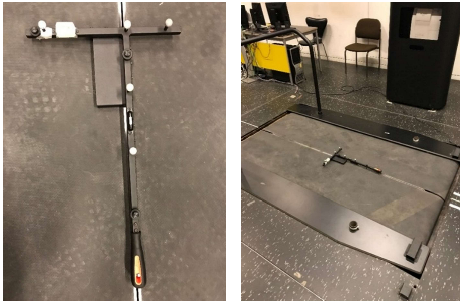
Figure 43. Images of the calibration wand in place at the centre of the treadmill to define the orientation of the global coordinate system.
