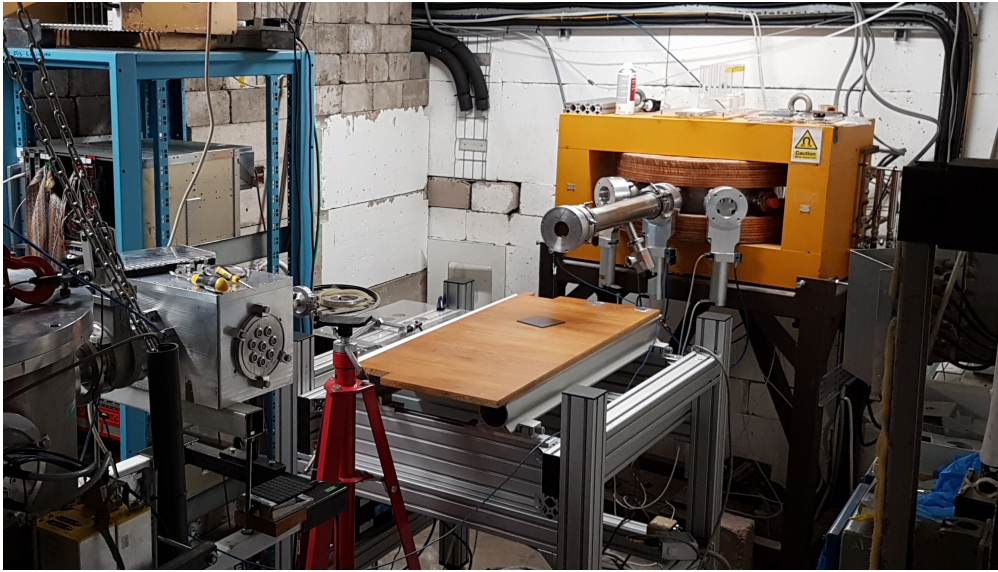
Figure 2.13 – Dedicated experimental room with height adjustable table behind the final collimator for studies with the LHCb VELO detector modules.
