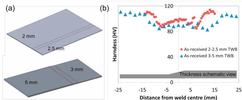
Fig. 1. Schematic of the FSWed 2.0-2.5 and 3.0-5.0 mm blanks and (b) hardness profiles of the corresponding TWBs.
