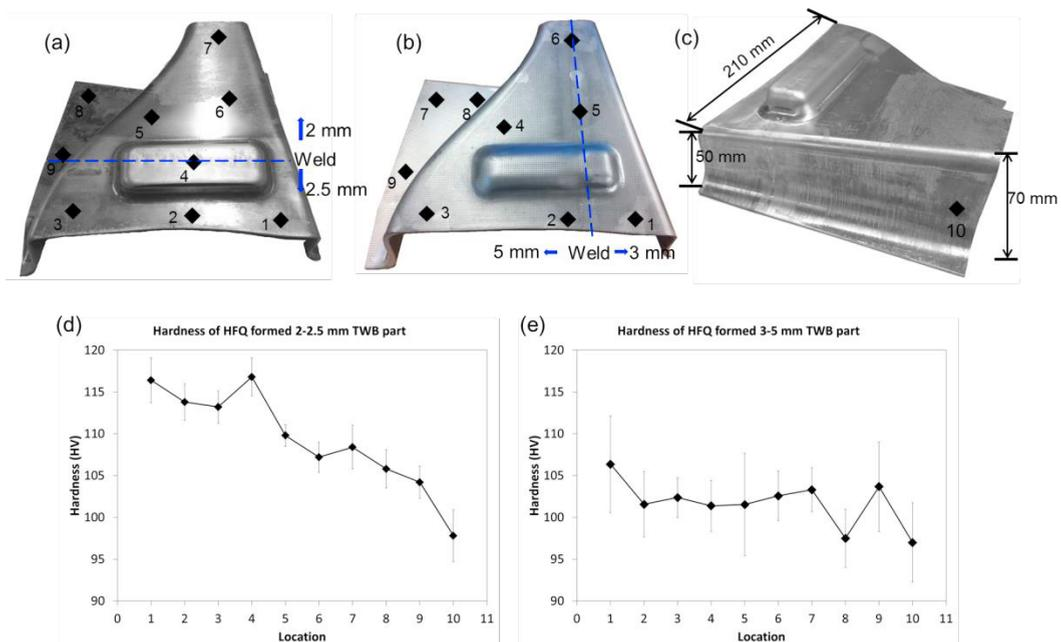
Fig. 2. HFQ® formed parts of (a) 2.0-2.5 mm TWB, (b) 3.0-5.0 mm TWB and (c) dimensions of the part, and hardness profiles for the (d) 2.0-2.5 mm and (e) 3.0-5.0 mm TWB parts.
