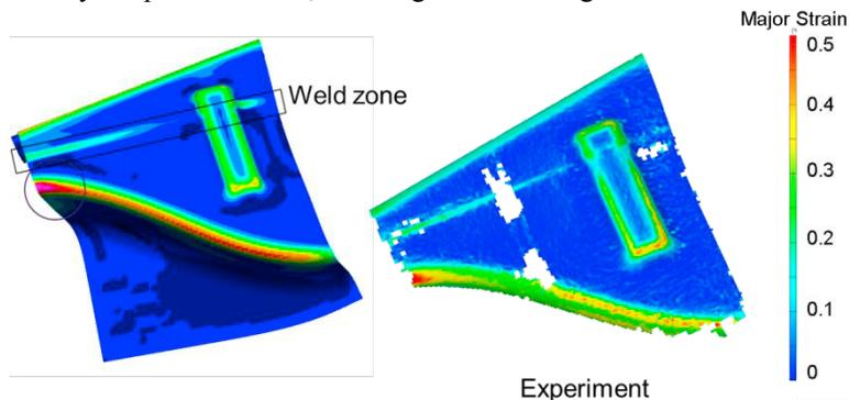
Fig. 4. Comparison of strain distributions in the 3.0-5.0 mm TWB between (a) simulation and (b) experiment.
