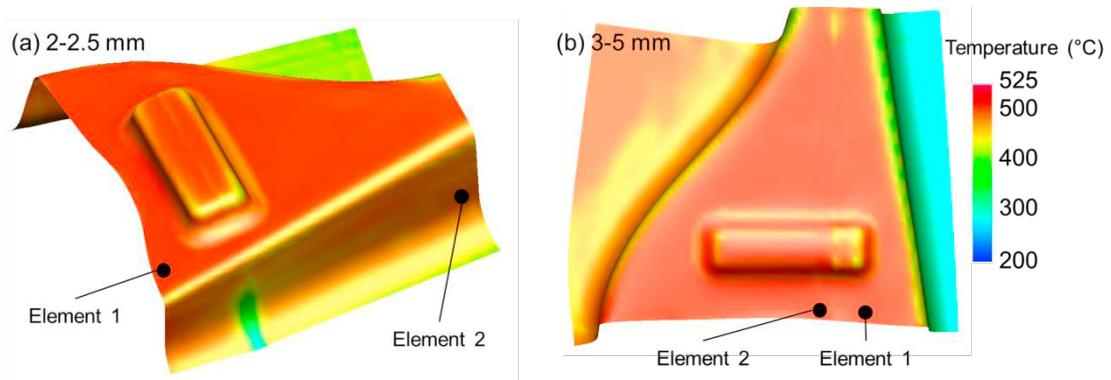
Fig. 5. Predicted temperature distribution during quenching of the formed parts: (a) 2.0-2.5 mm and (b) 3.0-5.0 mm.
