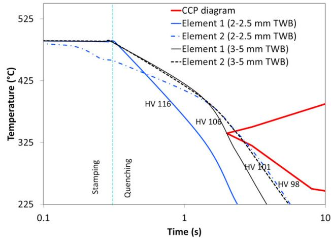
Fig. 6. CCP diagram of typical AA6082 [3] and temperature history for the selected elements in Fig. 5.
