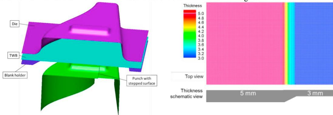
Fig. 3. (a) Pam-Stamp simulation model and (b) shell elements for the 3.0-5.0 mm TWB with thickness schematic view.
