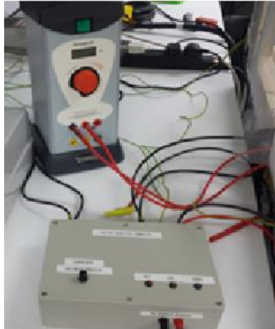
Figure 5-18 DC and AC power supply
