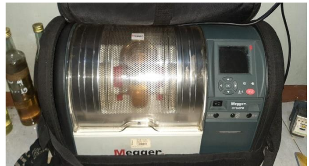
Gambar 1. Megger OTS60PB dielektrik breakdown testing
