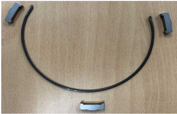
(a) C-spring of synchronizer
