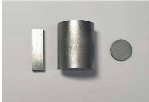
Figure 5.19. Typical dense pellets obtained by SPS with a diameter of 13 mm and a height of ~16 mm (center) and the specimens cut for measuring electrical (left, a bar with a length of ~15 mm) and thermal transport properties (right, a disk with a diameter of 8 mm) along the pressing direction of SPS.
